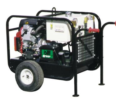
This power unit features a 22 HP Honda OHV gas engine, extended run fuel tank, extra oil cooling and easy handling. It is available with a fixed displacement gear pump or pressure compensated piston pump. Great for continuous duty applications powering our pumps or other hydraulic tools and equipment. Variable speed throttle controls hydraulic output.
