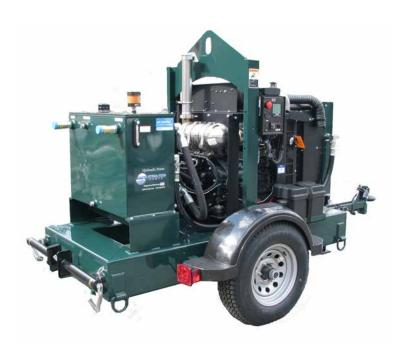
This popular unit features a Deutz diesel engine and pressure compensated hydraulic pump for maximum versatility and enhanced performance when driving submersible pumps or other hydraulic equipment.
