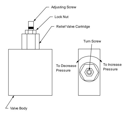
Relief Valve Pressure Adjustment
